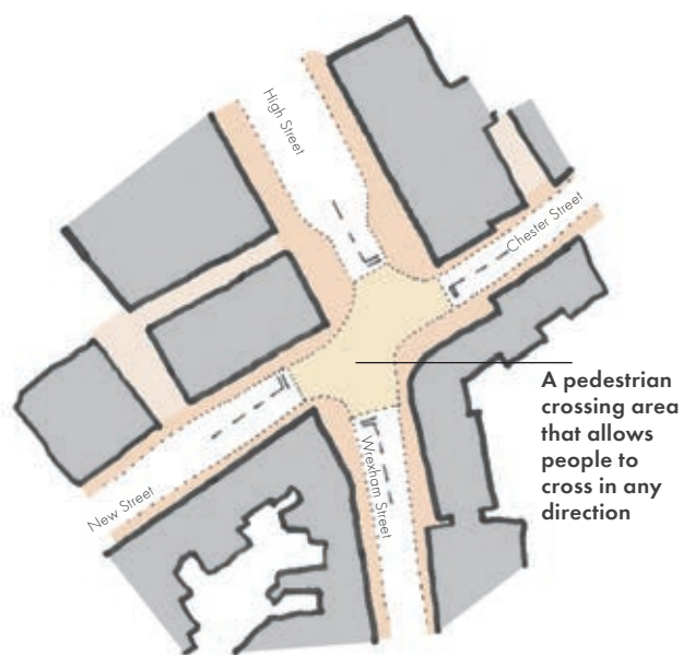
The Cross: an indicative design for the junction with a wide crossing area allowing pedestrians to cross diagonally, stopping traffic in all directions. The junction of Earl Road, King Street and High Street could also be treated in this way. At this stage, these are not formal proposals but indicative ideas.
