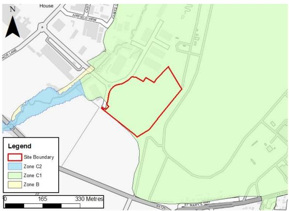
Figure 2-4 DAM mapping at site PE1.1
