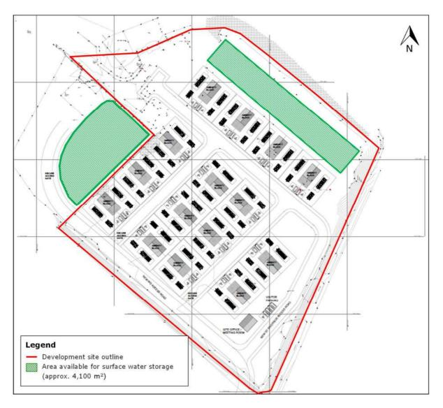
Figure 9: Preliminary Surface Water Drainage Layout
