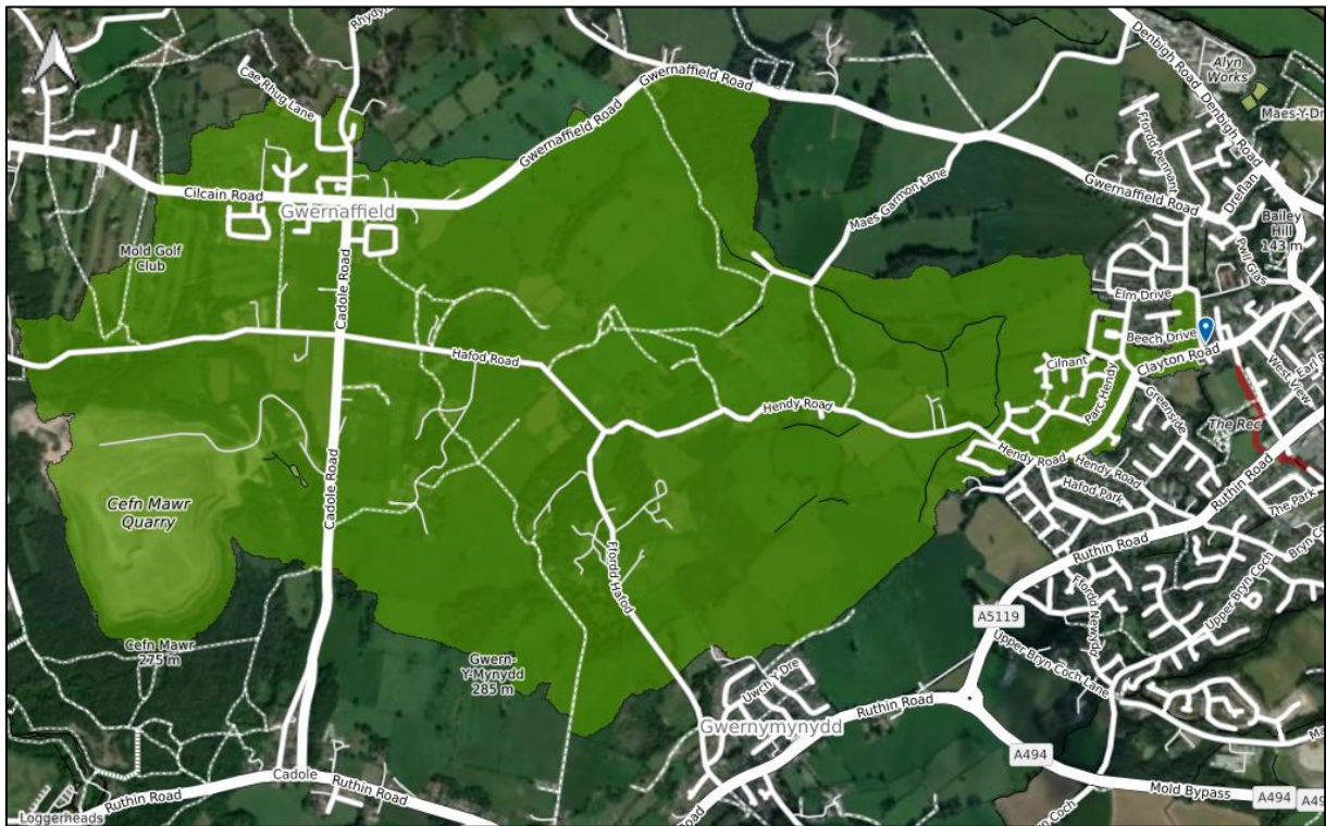
Figure 8 – Maes y March, Ash Grove, Clayton Road, Nant Garmon and Y Coetir Area Contributing Watercourse Catchment (source: SCALGO)
