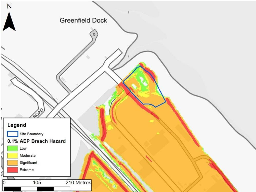
**Figure 4-10 Modelled hazards for the 0.1% AEP breach scenario**
