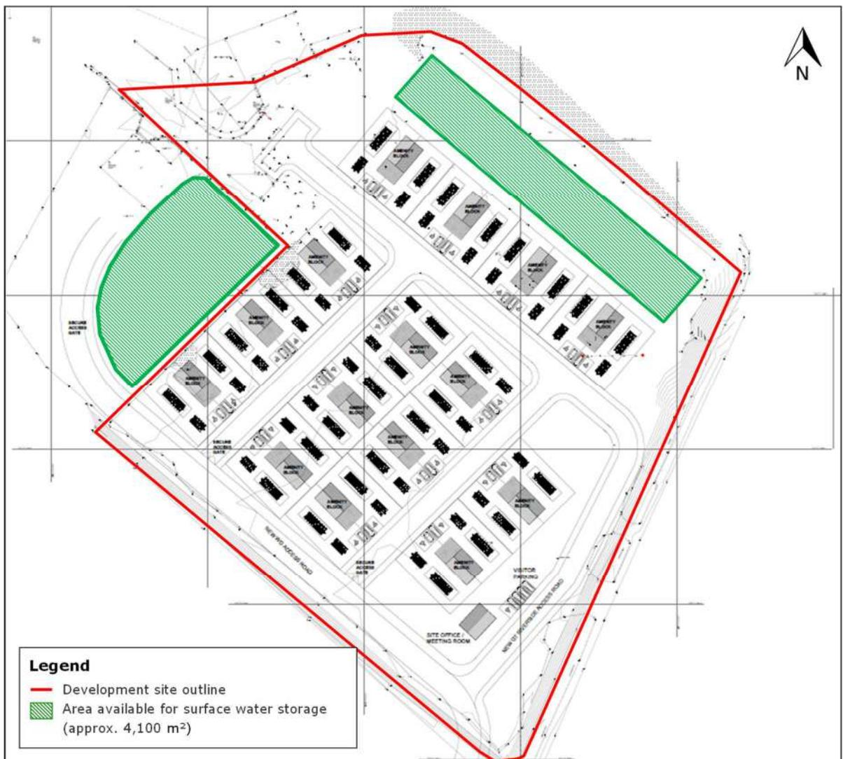
**Figure 9: Preliminary Surface Water Drainage Layout**
