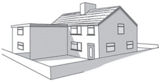
Figure 6 Unacceptable rear extensions
